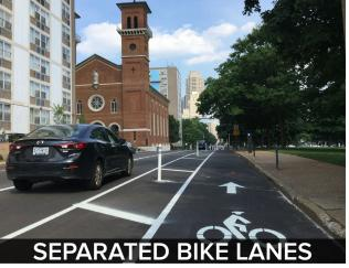
A separated bike lane is an exclusive facility for bicyclists that is located within or directly adjacent to the roadway and that is physically separated from motor vehicle traffic with a vertical element.
