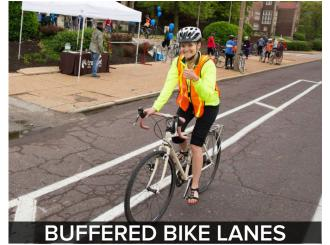
Buffered bike lanes are standard or conventional bicycle lanes paired with a designated buffer space separating the bicycle lane from the adjacent motor vehicle travel lane and/or parking lane.
